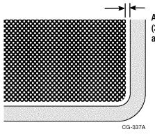
ALWAYS cut a 1/8" to 1/4" (3 to 6 mm) margin completely around the film.
